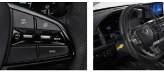
Steering wheel mounted cruise control Rake & reach telescopic steering wheel Tilt control of steering wheel angle switches
