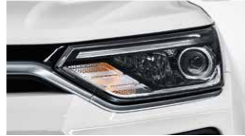
Projection headlamps with bulb-type turn signal lamps
