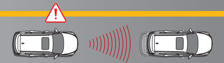
Front Vehicle Start Warning (FVSW) FVSW attracts driver's attention with a visual pop-up alert and audible sound when the vehicle directly in front is pulling away.
