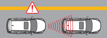
Safety Distance Warning (SDW) SDW calculates the distance to the vehicle in front and warns the driver when a safe distance is not maintained.
